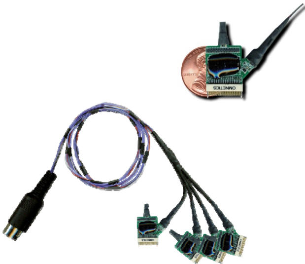
128 channel headstage system with a 6 wire cable (uses 4, 32 channel multiplexer headstages)
